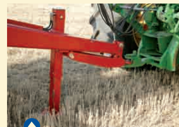
Drawbar height is hydraulically adjustable to suit tractor hitch (9 positions) 6.3m and 8m
